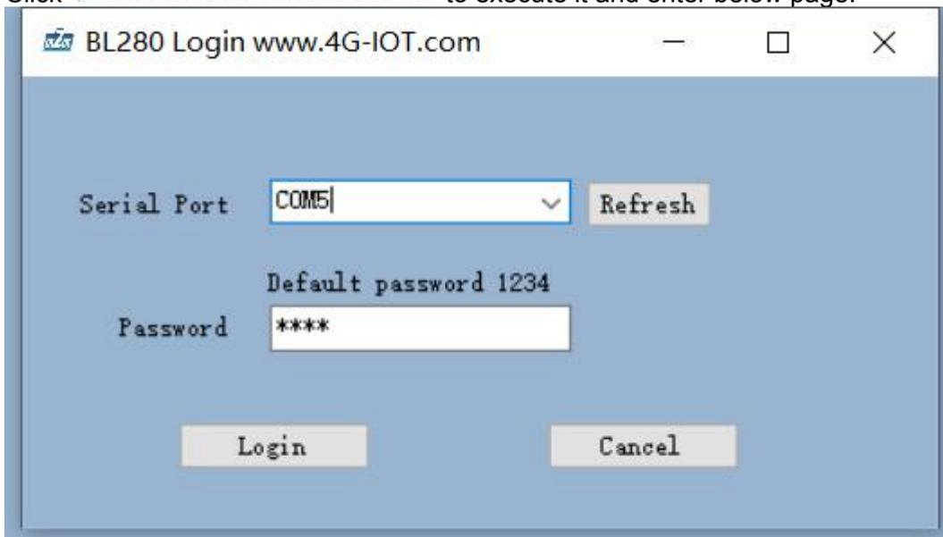
Select connected serial port  , input password (default is 1234 and it's filled automatically), click login to enter below main page. If login is not successful, please check USB connection, password and port number.
